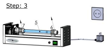
Lift the lamp (position 5) out of lamp clip A (position 6) and lamp clip B (position 7)
