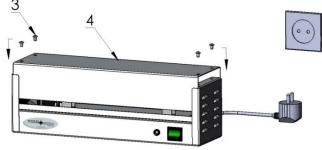
Attach the lid (position 4) and install the four screws (position 3)
