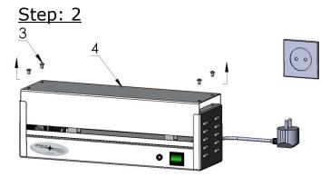
Remove the four screws (position 3) and remove the cover (position 4)
