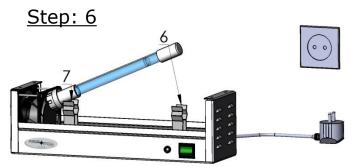
Push the lamp (position 11) down into lamp clip B (position 7) and lamp clip A (position 6)
