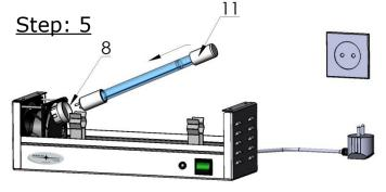
Insert the new lamp (position 11) into the socket (position 8)
