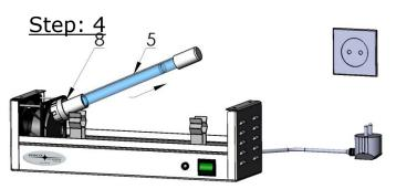
Pull the lamp (position 5) out of the socket (position 8)
